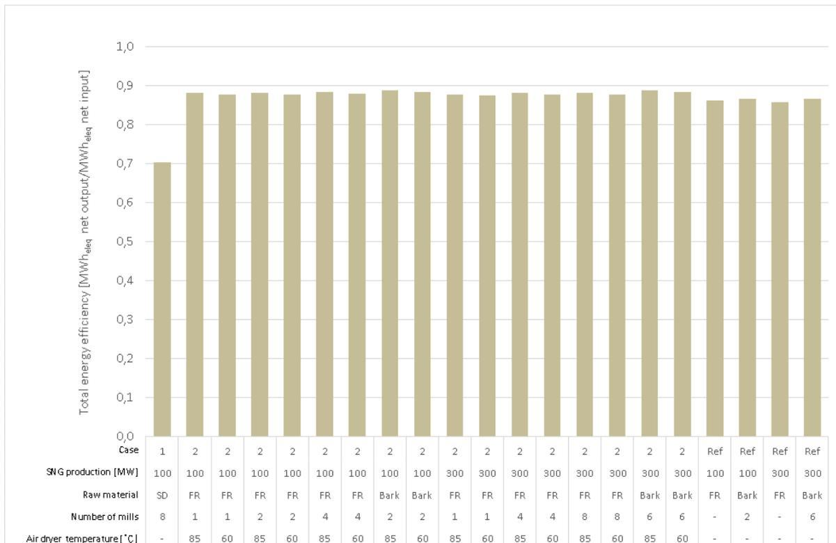
**Figure 15. Total energy efficiency ( $MWh_{elec}$  net output/ $MWh_{elec}$  net input).**
