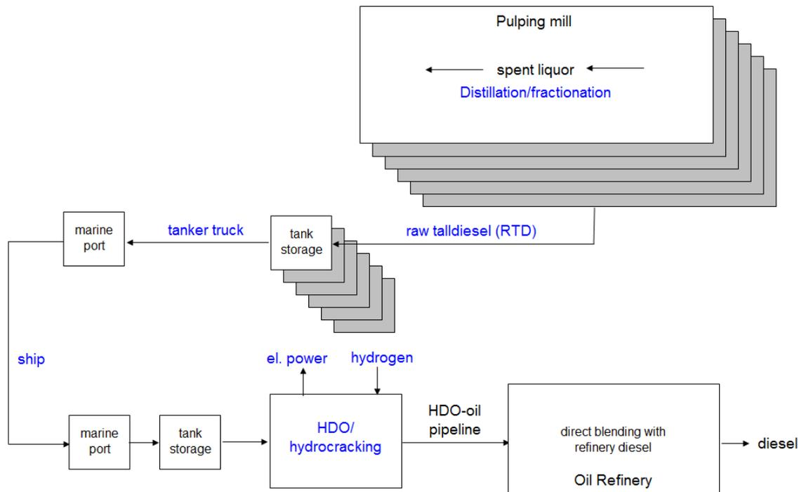
**Figure 14. General representation of HDO-oil production. In this study, the tall oil is assumed to be shipped directly to the HDO plant (i.e. no tanker truck needed).**
