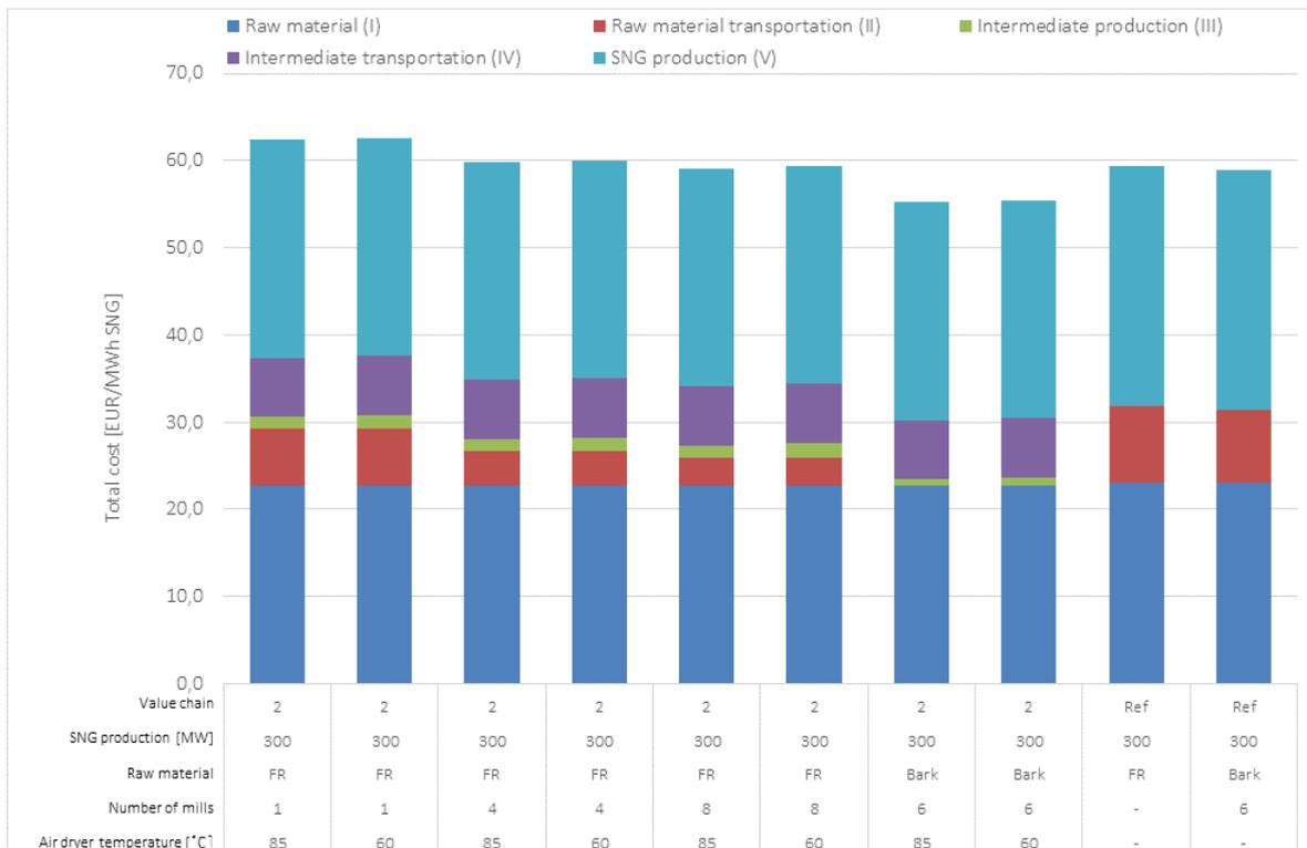
**Figure 18. Total cost for SNG (EUR/MWh) for the cases with an SNG production of 300 MW.**
