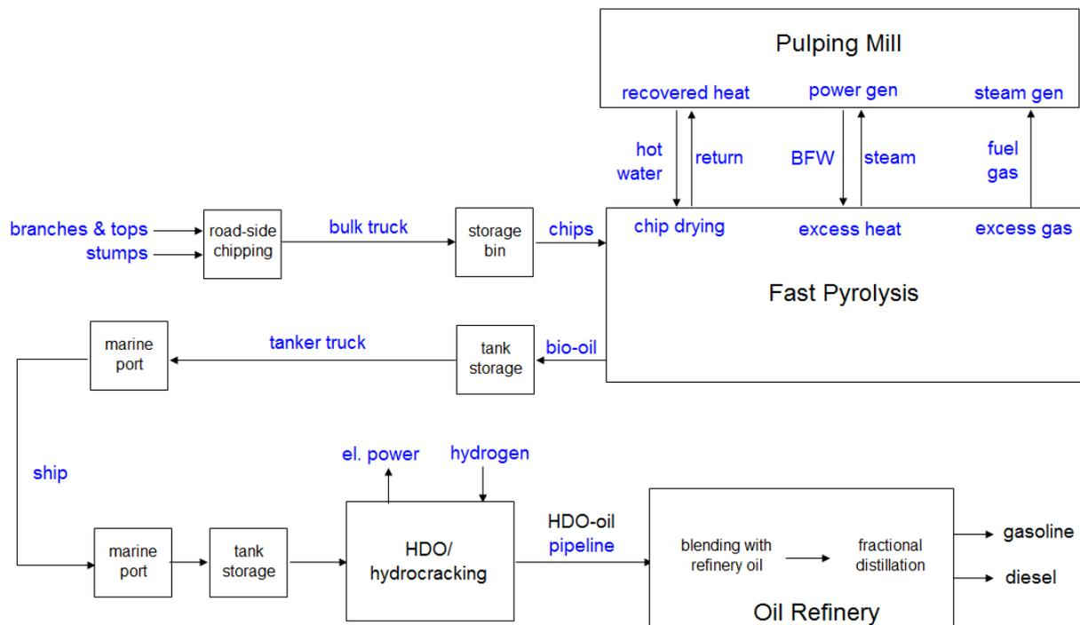
**Figure 11. General representation of HDO-oil production. In this study, the bio-oil is assumed to be shipped directly to the HDO plant (i.e. no tanker truck needed).**
