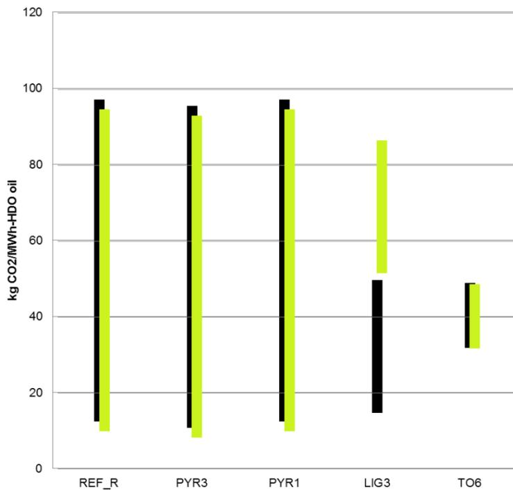
**Figure 21. Sensitivity analysis CO<sub>2</sub> emissions. Green bars: Nordic electricity mix (102 kg<sub>CO2</sub>/MWh), black bars: Swedish electricity mix (25 kg<sub>CO2</sub>/MWh). Top of the bar: H<sub>2</sub> from methane reforming, bottom: H<sub>2</sub> as byproduct from refinery.**
