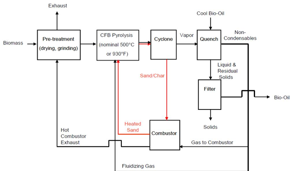
**Figure 8. Illustration of the fast pyrolysis process (Jones et al. 2009).**
