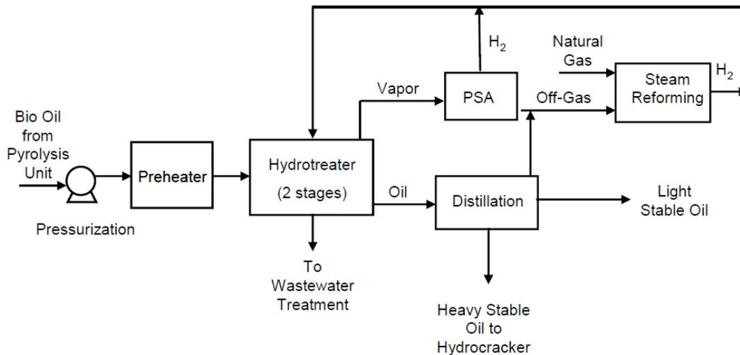
**Figure 10. Illustration of the HDO process (Jones et al. 2009).**
