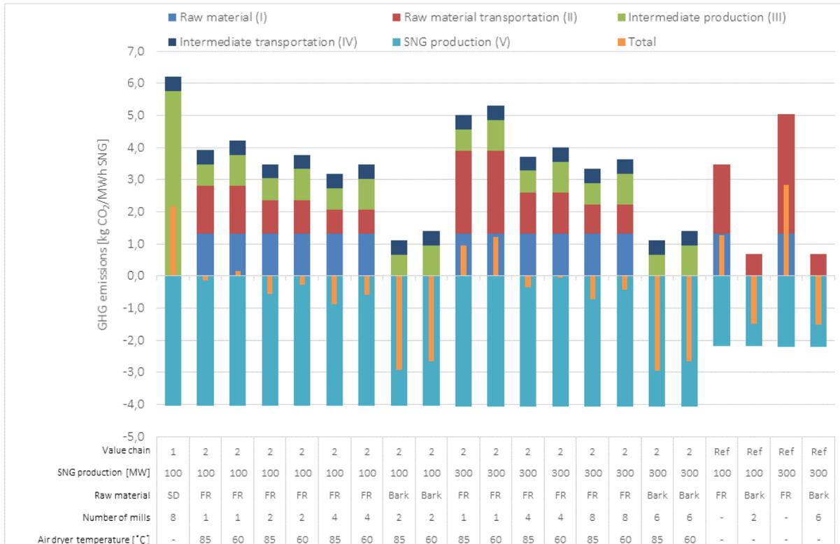
**Figure 16. Change in CO<sub>2</sub> emissions (kg CO<sub>2</sub>/MWh). Usage of bio-SNG is not included. Negative values indicate a decrease of CO<sub>2</sub> emissions.**
